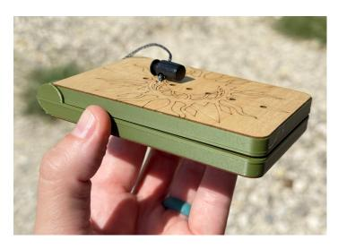
To store the sundial, simply close it up. You can use the cord lock to keep it closed; just snug it up to the top of the device. If you leave the cord in the hole for your location then it's a 2-second job to open it up and get a time reading. And of course, you also have a compass, so you won't get lost!
