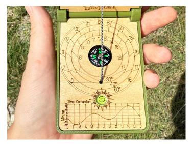
Here, it reads 14:00 Solar Time, which is about 15:36 CDT here at 30° latitude (Central Texas) on the 1st August. We're adding six minutes for the time correction (you always subtract the minutes, so here we're subtracting a negative number, hence adding it) and I'm about 30 minutes offset in my time zone. And it's Summer Time. So 6+30+60 = 96 minutes difference to Solar Time.
